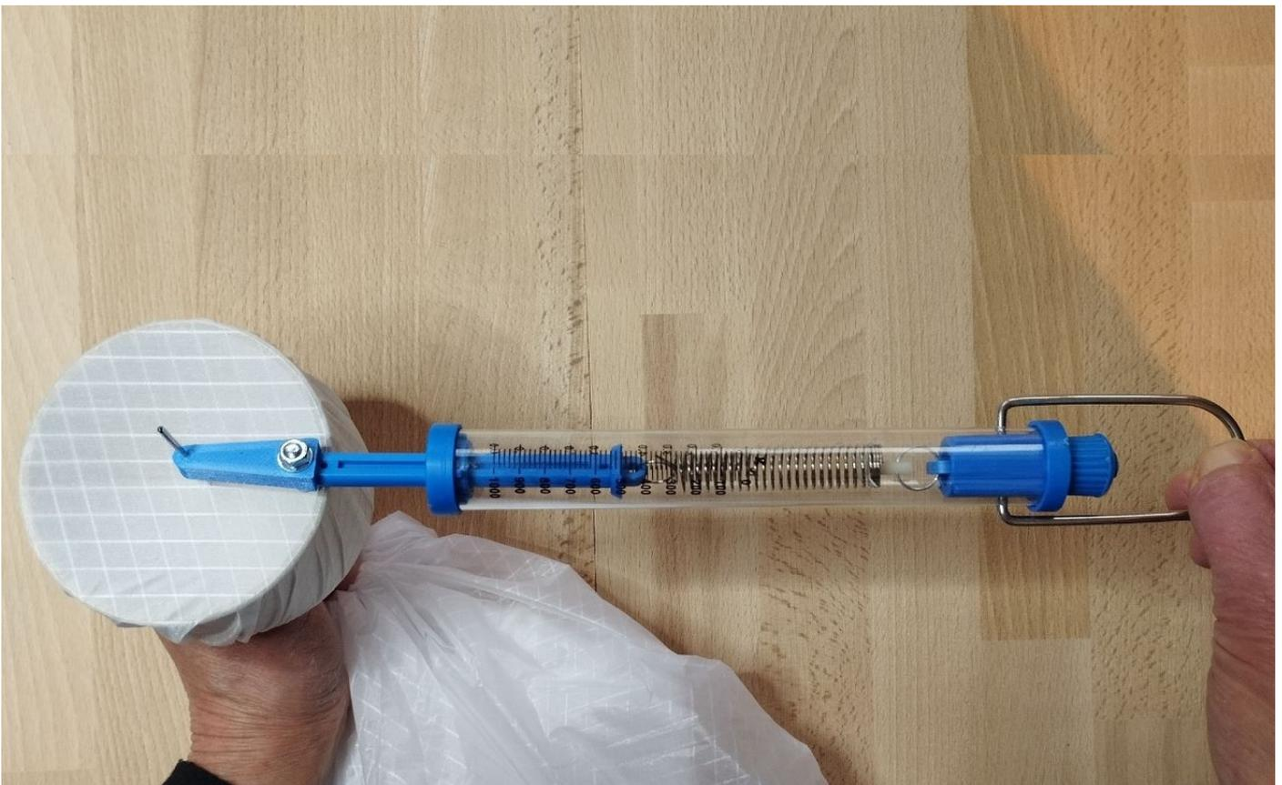
In private use, the measurement of the tear strength does not replace the prescribed service or check of your glider. The glider must be checked regularly by an authorized service center according to the manufacturer's instructions and local regulations. In addition to the tensile strength of the canopy, this person will also check the porosity and damage of the canopy, as well as the line lengths and their breaking load.
